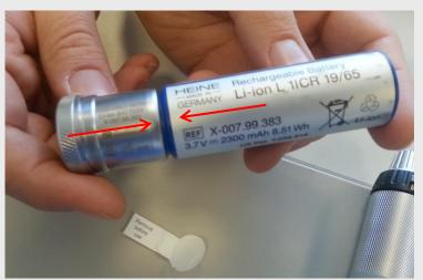
Reassemble bottom cap and battery, an audible click confirms the proper connection.
