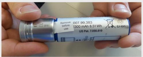
Remove battery completely from handle.
